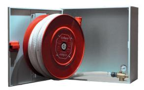
Fire hose cabinet Ø25 mm according to EN 671-1 standard with 20 m of semi-rigid hose manufactured according to EN 694.
