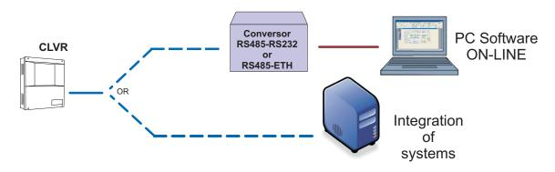
Example of connection for MODBUS functionality
