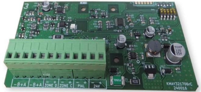
Up to a maximum of 10 conventional alarm call points can be installed on the strip of “Zone C”. The “Zone D” strip allows a maximum of 32 temperature detectors (A30XT, A30XV) or 32 components between smoke detectors (A30XH, A30XHS) and conventional alarm call points. Both strips supervise the line using a 4K7end-of-line resistor. It thus indicates the status of the open line, crossed line, detector alarm or alarm call point alarm.
