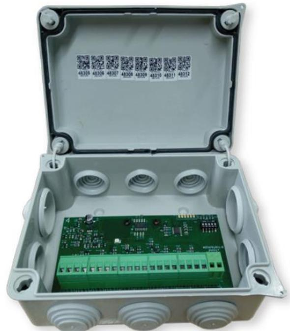
Using pin 2 of the configuration microswitch we will select the type of event that the module will send to the control panel: ON Fault and OFF Alarm.
