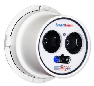
The DLRCM detector is a linear optical smoke detector with a motorised self-regulating microprocessor, which bases its operation on the interaction between the smoke present in an environment and an infrared beam emitted by the device and reflected by an optical reflector.
